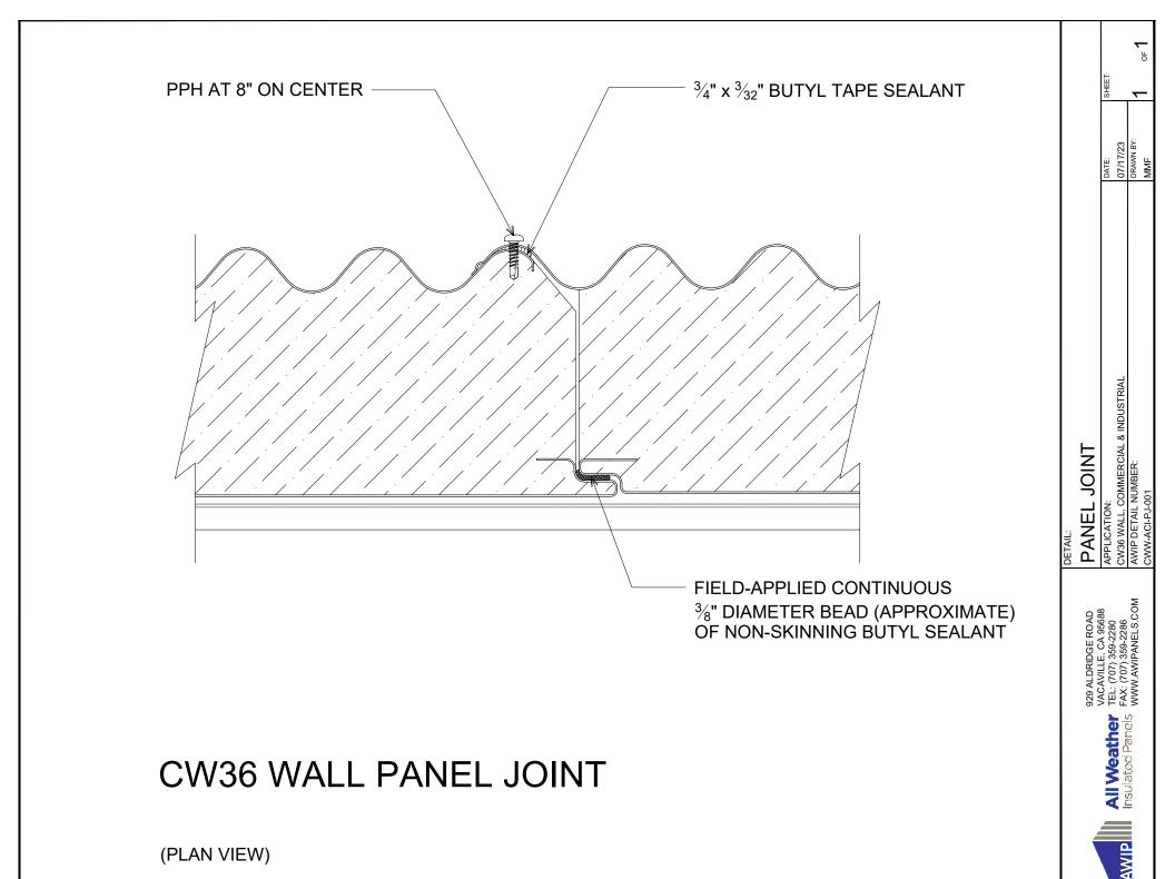
NOTE: FASTENING SCHEDULE MAY VARY DEPENDING ON SPECIFIC APPLICATION. INTERMEDIATE WALL FASTENING EXTERIOR INTERIOR **SECONDARY FRAMING** "CW-02" CONCAVE BONDED (NOT BY IMP SUPPLIER) SEAL WASHER W/  $\frac{1}{4}$  - 14 x \_ TEK 3 FASTENER W/ WASHER INTO SUPPORT MEMBER (SEE WALL FASTENING LAYOUT)
