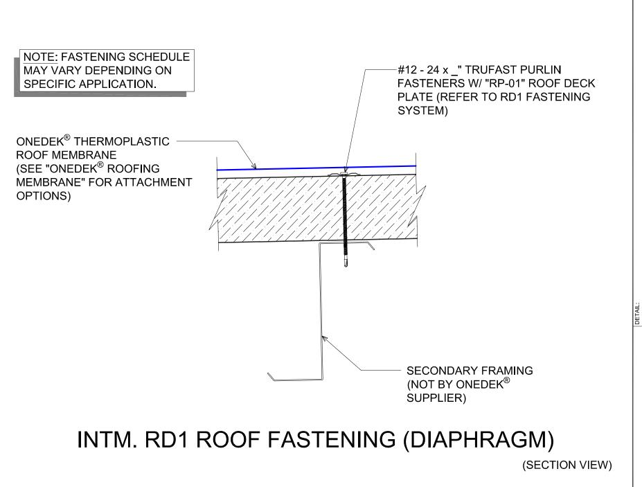
INTERMEDIATE RD1 ROOF FASTENING (DIAPHRAGM)
