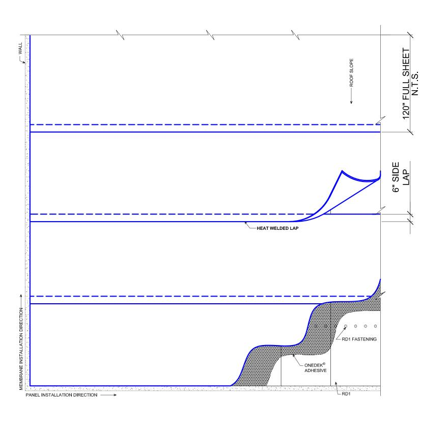
NOTE: ULTIMATE WIND UPLIFT LOAD: 135 PSF. ALLOWABLE WIND UPLIFT LOAD: 67.5 PSF.
