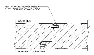
NOTE: FILL WARM SIDE FEMALE JOINT WITH 3/8" DIAMETER BEAD (APPROXIMATE) OF NON-SKINNING BUTYL SEALANT (DO NOT UNDER-FILL).
