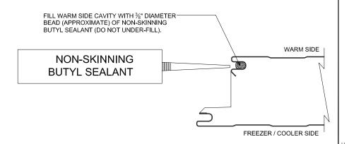
SEALANT PLACEMENT AT PANEL JOINT (PLAN VIEW - LINER; SECTION VIEW - CEILING)
